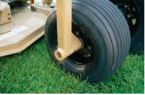
Gauge wheels feature bolt in spindles for ease of replacement, and 18" tires leaving a light weight footprint.
